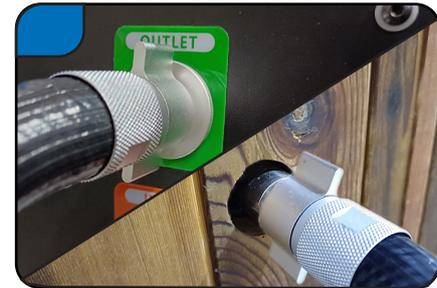
Next, using the second hose, thread one end onto the OUTLET on the rear of the chiller. Then thread the other end of the hose onto the BOTTOM connection point on the Apollo. Excess hose should be coiled up and placed between the chiller and the ice bath to prevent becoming a trip hazard.
