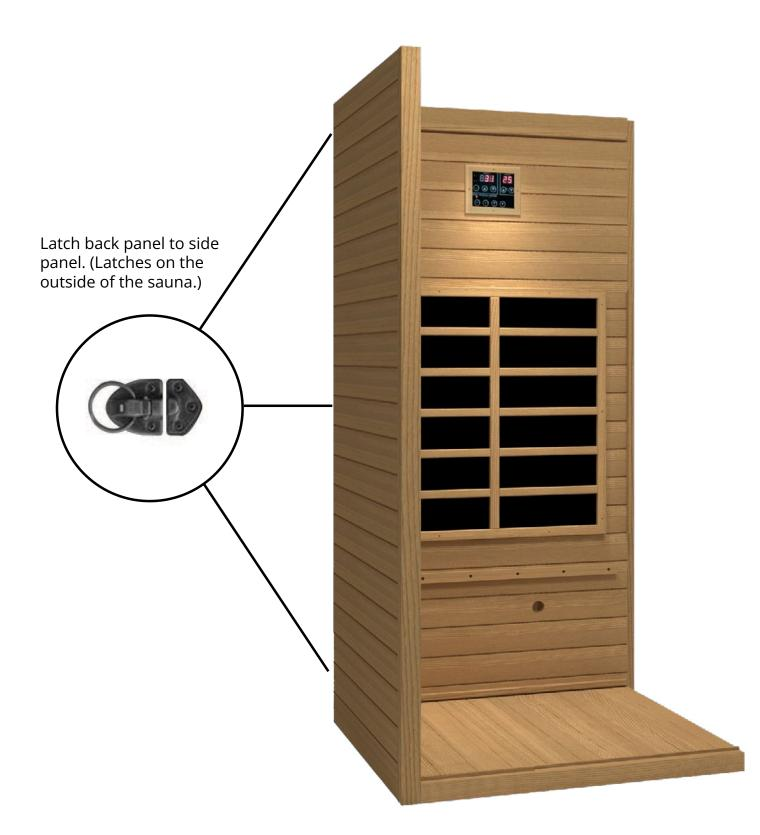
**4.** Place the remaining side panel up against the floor panel and latch to the back panel.
