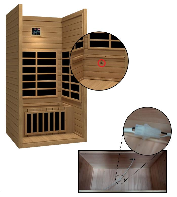
6. Place the Bench Seat inside the sauna on the provided supports, be sure to push the bench seat firmly against the rear wall panel. Screw the bench seat into the left and right supports using 2x 4\*40mm screws. There are two pre drilled holes located at the back of the Bench Seat to guide the mounting screws.
