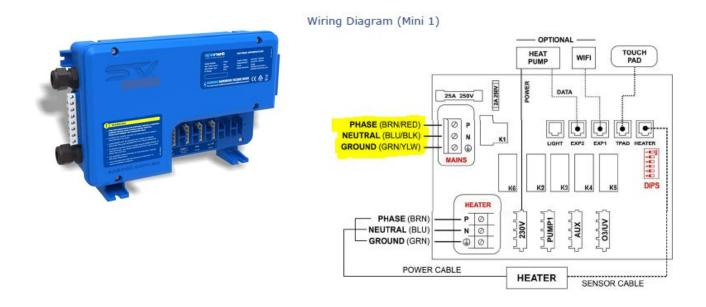
Using the topside control panel, the OEM menu must be accessed and L.SHD setting must be set to the value of '2' - follow below instructions.
