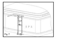
**STEP 7:** Safely stand to side and remove the "Locking Cable" and allow the cover support frame to pivot outwards. (Fig. 7)
