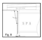
**STEP 8:** Slide the cover lifter support frame either up or down to allow the spa pool cover to slide evenly along the top of the spa lip into the cover basket. (Fig. 8)
