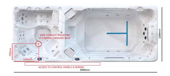
The Columbus - Advanced Swim uses the SpaNET SV Mini 2 Controller with a SpaNET SV2 Touchpad (labelled SV-Smart) in the spa zone, and a SV3 controller and Touchpad in the swim zone.
