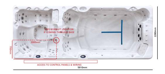
The Jupiter - Pro Swim uses the SpaNET SV Mini 2 Controller with a SpaNET SV2 Touchpad (labelled SV-Smart) in the spa zone, and a SV4 controller in the swim zone.
