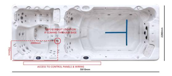
The Jupiter - Advance Swim uses the SpaNET SV Mini 2 Controller with a SpaNET SV2 Touchpad (labelled SV-Smart) in the spa zone, and a SV3 controller in the swim zone.
