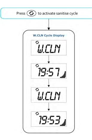
Whilst the cycle is running the display alternates between the W.CLN (water clean) title screen and the minutes remaining in the cycle (refer above).
