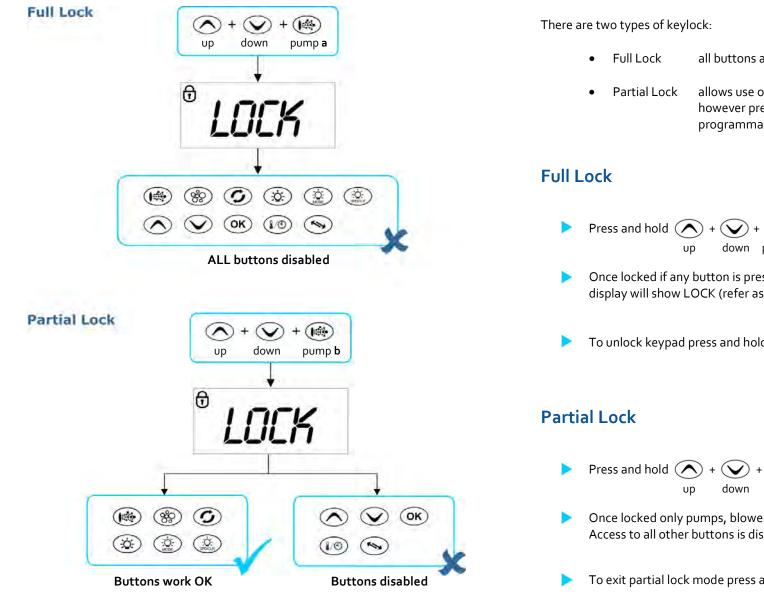
The keypad buttons can be locked to prevent accidental key presses or to limit access to certain controller functions. This feature is particularly helpful when spa covers are used or where children are present.
