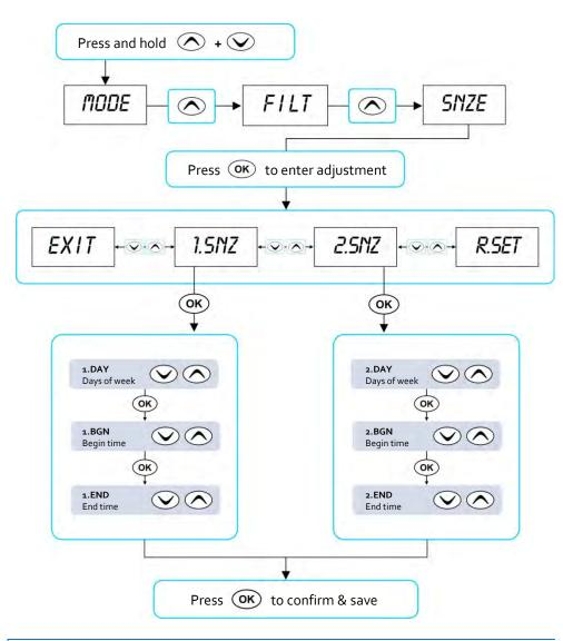
Accessed via the Setup Menu, Sleep timers are a very handy feature that enables the user to stop all spa activity during certain times of day or night. While the controller is sleeping NO automatic heating or filtration maintenance will occur, however the spa can still be operated by manual use without the need to adjust sleep time settings.
