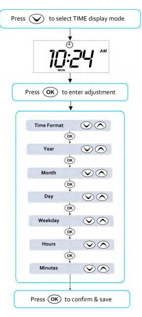
Be sure to set the date and time before operating the spa. Vital functions such as filtration, sanitisation cycles and power saving settings depend on the time and date being set correctly.
