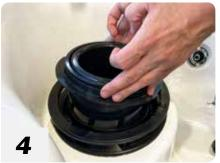
Remove the filter core.
