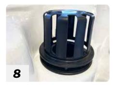
Replace the basket, filter core and lid in order, turning the lid clockwise to secure it.
