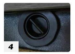
Check the external drain valve is in the 'flow-locked' position (retracted) with the inner twist cap screwed in tight.
